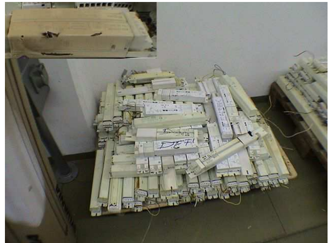
Image: Electronic ballast failures at Swiss Federal Institute of Technology, Zurich within one year.
